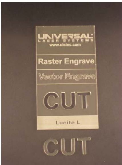
Figure 1. Raster Engraving, Vector Engraving and Cutting LuciteLux™ in a single laser processing operation.
