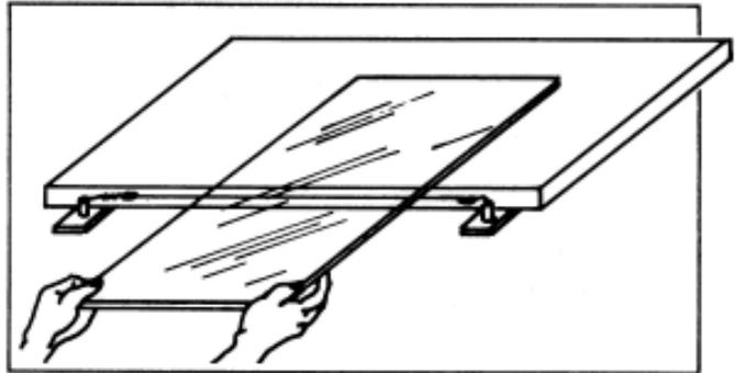
Heat the material until it bends easily. Experience will teach you how long to heat each part. Don't overheat or lay ACRYLITE FF sheet directly on the heating element - doing so will blister and/or mark the sheet.
