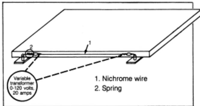
To bend ACRYLITE® FF acrylic sheet up to 1/8" (3mm) thick, the most commonly used piece of equipment is a straight nichrome wire resistance heater. The unit functions similarly to a household electric toaster by passing electricity through a wire.
