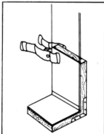
Use a cooling jig like the one shown at left to assure that your bend is at the proper angle and to prevent the piece from "springing back" into its original shape. This is an all-purpose jig for 90° bends - you can modify it to suit the part. A cooling jig which exposes both sides of the heated
