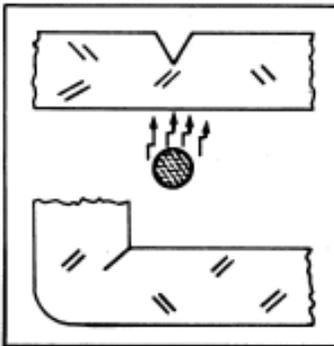
For sharp line bends with no deflection, it is a good idea to v-groove the sheet, as shown at left. Use a v-rabbit router bit or a table saw, making two opposed 45° cuts. V-grooving the sheet reduces the material cross section at the point of bending, reducing stresses and
