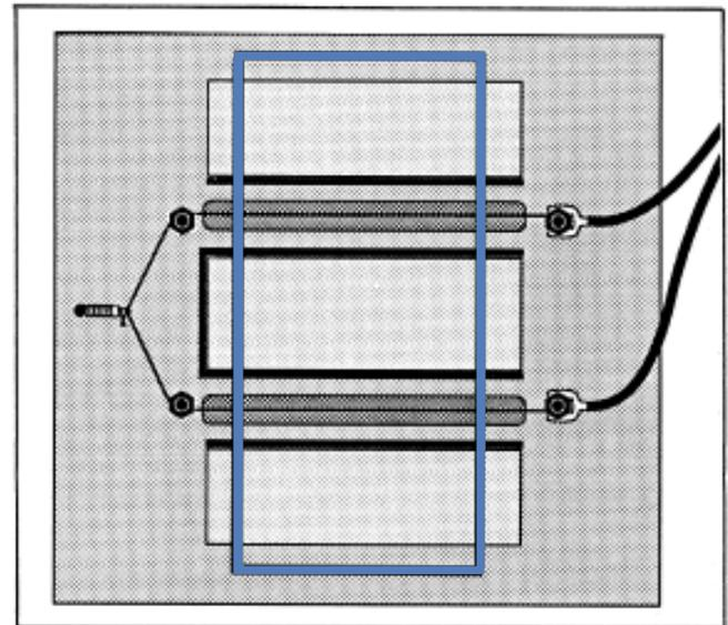
To perform multiple line bends, modify the heater as shown above. Where the wire joins the spring, include an insulation ring. Raise the unit's base so convection air from below flows through slots routed in the base as shown.
