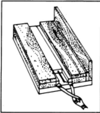
To heat sheet thicker than 1/8" (3mm), use a tubular-rod heater with a heating rod like the heating element of an electric stove. Power the heater with a variable transformer. Place a reflector, preferably of split aluminum conduit for its good reflectivity,
