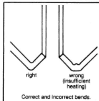
When line bending with only one heating element, be sure to bend away from the heated side. For example, if the nichrome wire is on the bottom, bend upwards.
