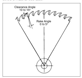
For gang cutting of stacked sheets, a saw blade whose teeth have increased radial clearance is recommended. This clearance will reduce carbide/plastic contact on the sides of the teeth and, therefore, reduce heat generated by friction. Use ACRYLITE FF sheet masked with polyethylene masking where possible when gang cutting; the polyethylene masking acts as a lubricant.
