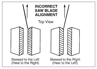
Run-out (or wobble) of the saw arbor and blade collar should be essentially zero. Total run out, including the saw blade, should be less than 0.002". A simple dial indicator to measure the run-out can be purchased from industrial hardware suppliers such as Sears.
