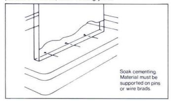
Leave the piece in the solvent 20 seconds for thin sheet and 30 seconds for relatively thick material. The time varies for different solvents and bond strength requirements—experience will help you plan the correct dipping time. Consult CYRO's technical group (last page of this brief) if you need advice.
